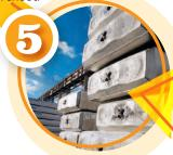
The pieces are then melted and cast into ingots.
