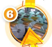
Ingots are then hot and cold rolled into coils of can sheet.
