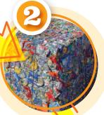
Used beverage cans (UBCs) are then crushed and flattened into bales.
